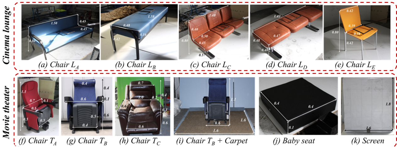
Figure 2. Photographs of combustibles selected in cinema lounge and movie theater (the unit of scale shown in the photos is m).
