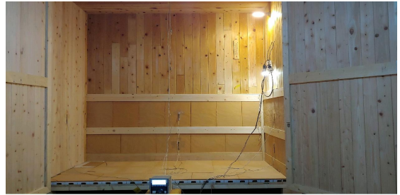
Fig. 3 Measurement of air temperature and wall surface temperature inside the ocher jjimjilbang
