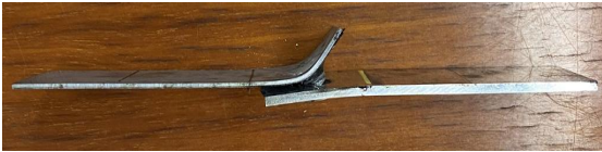
Fig. 5 Appearance of Hybrid SPR tensile shear test piece
