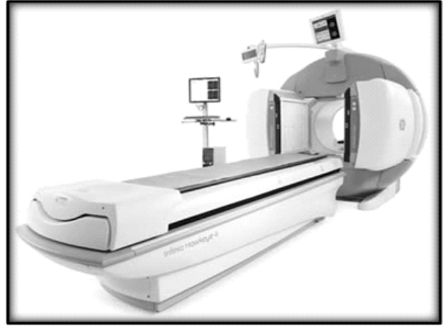
Fig. 1. The \gamma -camera named GE INFINIA(GE Healthcare, USA) is used.
