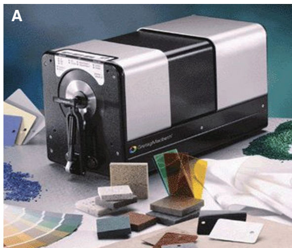
Fig. 1. (A) A spectrophotometer (Xrite Benchtop Spectrophotometer Color i5, Xrite, USA), (B) The CIELAB color space (CIE L^*a^*b^* , or abbreviated as Lab color space).
