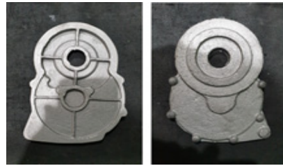
Fig. 7. Casting products manufactured using Ib+W(0.05wt%)
