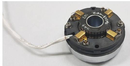
Fig. 7. Configuration of tachometer generator.
