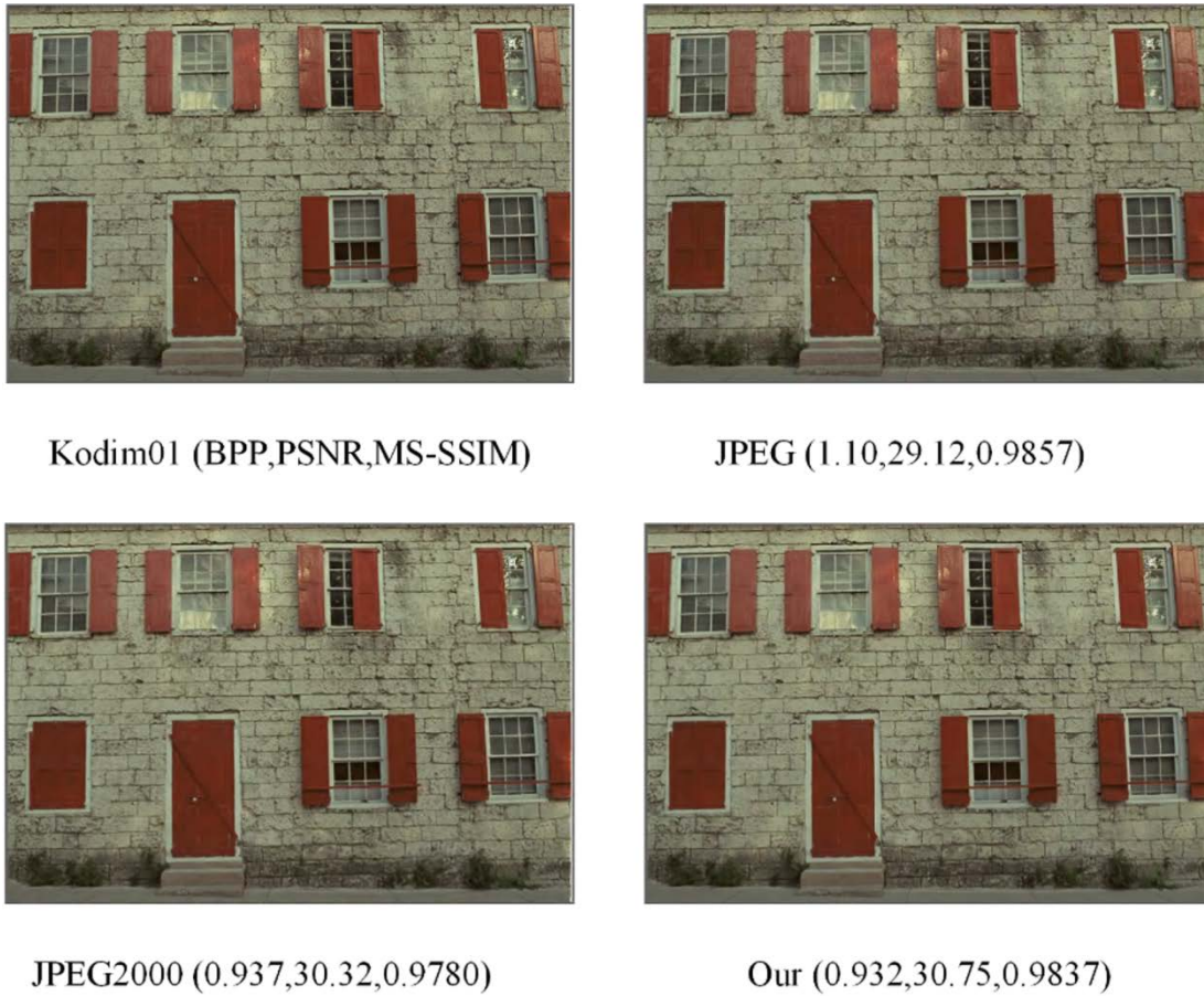
Fig. 3. Image produced by different compression systems at different compression rate. From the left to right: groundtruth, JPEG, JPEG2000 and Ours.
