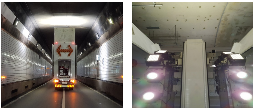
Fig. 3. Image-data collection vehicle (tunnel-lining scanning)
