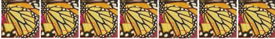
Fig. 4. Comparison of SR results on Butterfly by different methods (scaling factor s = 3 ), from left to right and from top to bottom: Bicubic, ScSR[13], ANR[17], ASCSR[33], SRCNN[26], ASR+LR[34], Proposed method.
