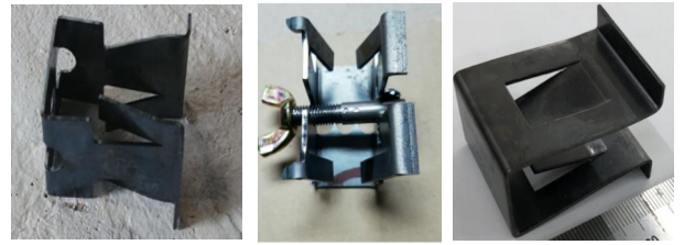
(a) Initial shape-1 (b) Initial shape-2 (c) Final shape Figure 4. Development process of clip-type binding implement
