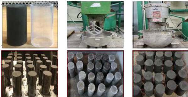
Figure 2. Specimen and mixer, curing process
