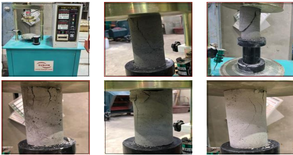
Figure 5. Compressive strength test method
