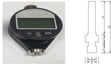
Figure 5. Improved type durometer
