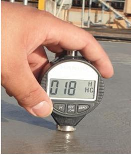
Figure 6. Measurement method of durometer
