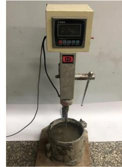
Figure 2. Proctor penetration resistance tester
