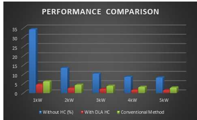
Fig. 15. Comparison of the inverter output THD with and without harmonic compensation method.
