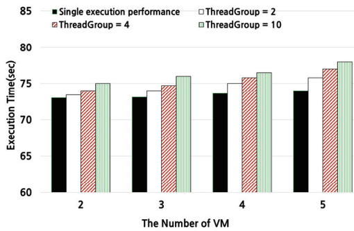
Fig. 5. Performance of GPGPU Operation According to the Size of the Thread Division
