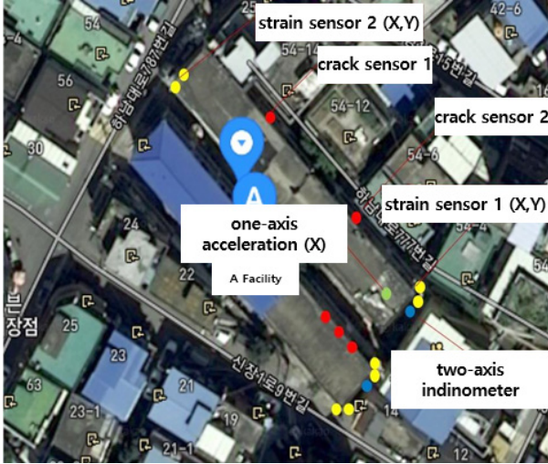
Fig. 3. A Facility Sensor Location
