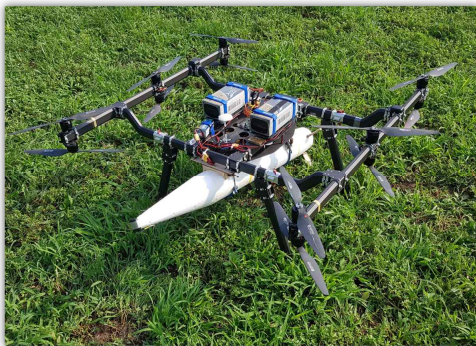
Fig. 6. Multirotor(dodeca) UAV as a mother ship and a guided munition mounted on the bottom side
