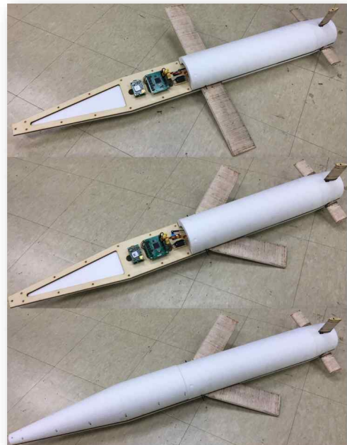
Fig. 2. Replica of guided munition made up of expanded polypropylene(body), plywood (skeleton), and balsa wood(wing, fin)
