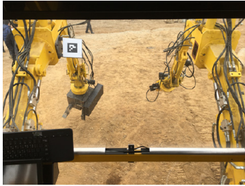
[Fig. 2] The dual hydraulic manipulators cover almost 40% of the front view of the operator, and only 60% information from the front view is provided to the operator
