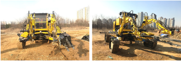
[Fig. 1] Our target application system is a 6 ton, dual-armed, and hydraulic robot system for reacting disaster sites
