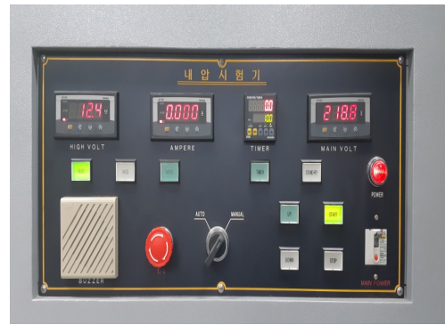
Fig. 14. AC Breakdown Voltage Equipment
