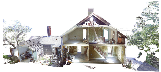
Figure 6. 3D laser scan data of a historic residence (Source: University of Florida Envision Heritage)
