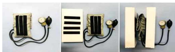
Figure 2. Measuring instrument for the pressure of hip adduction
