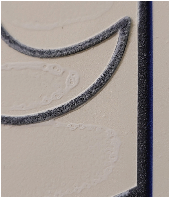
Fig. 8. Detailed photos of real samples of odor-ink applied swell papers
