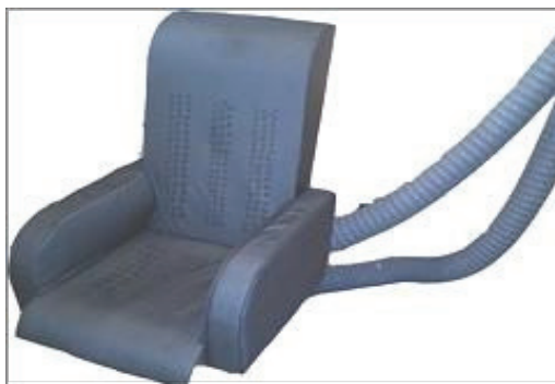
Fig. 1. Ventilation Seat applied air conditioning systems
