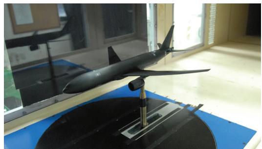
Fig. 11 CRM model in small low speed wind tunnel.
