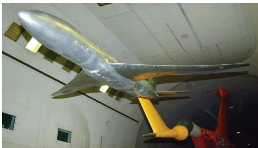
Fig. 3 The LRM model in S1MA wind tunnel[6].
