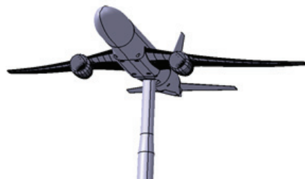
Fig. 7 CRM with Belly sting support.
