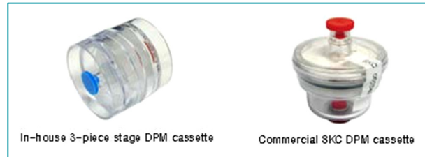
Fig 1. Preloaded quartz filter cassettes for DPM exposure monitoring.
