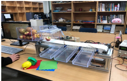
Fig. 6. Capture fruit with the Pi camera
