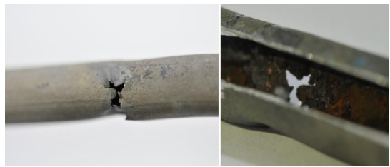
Fig. 6 An air line failure of the mix truck
