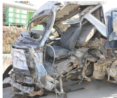
Fig. 2 Damage to the front of the mix truck
