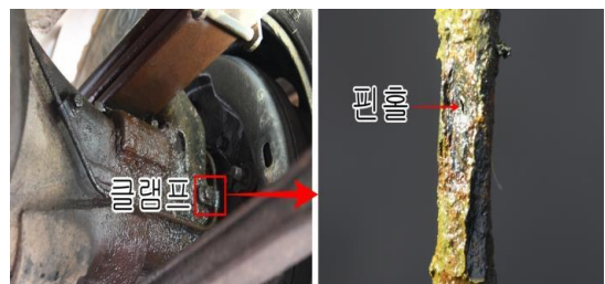
Fig. 10 A location of the oil leakage
