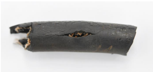
Fig. 15 A burst pattern of the flexible hose
