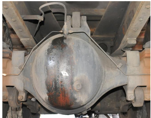
Fig. 17 An oil leakage on T type adaptor of 3rd axis
