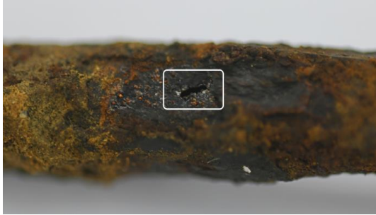
Fig. 11 A pin-hole and corrosion status of brake line
