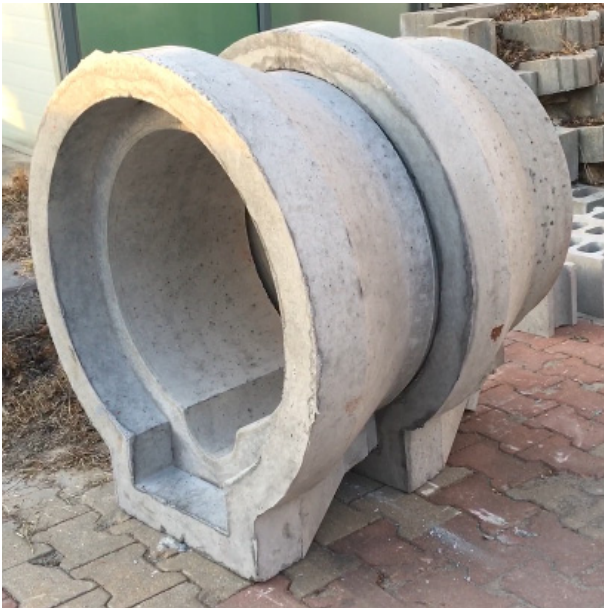
Fig. 8. Mock-up test of complex cross section concrete pipe.
