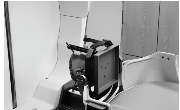
Fig. 2. Docking mechanism of LGK PFX PPS.
