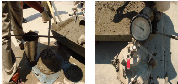
(b) Slump test
