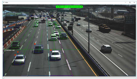
Fig. 3. Photograph of the image processing sensor which extracts the vehicles from the video image of CCTV.
