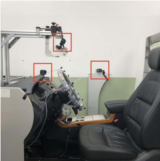
Fig. 1. Constructed virtual driving platform for driver image collection. Red squares indicate the camera placements.
