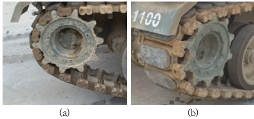
Fig. 4. Influence of tension between sprocket and track
