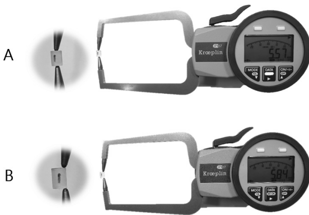
Figure 4. Measure the length of the specimen using a digital meter. (A) Inner diameter measurement, (B) Outer diameter measurement.
