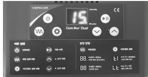
Figure 3. UV curing machine.
