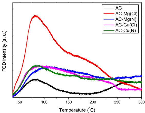
Figure 3. TCD intensity through NH<sub>3</sub>-TPD of samples.
