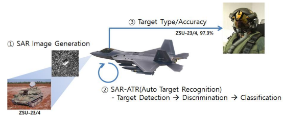
[Figure 1] Concept of operation for auto target recognition based on SAR image by using radar equipped on fighter jets
