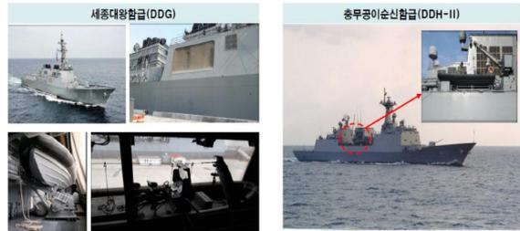
[Figure 11] Case of Mother Ship Mounted Small Boat
