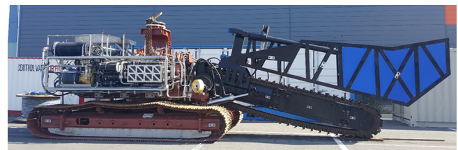
Fig. 1 Underwater construction robot URI-R
