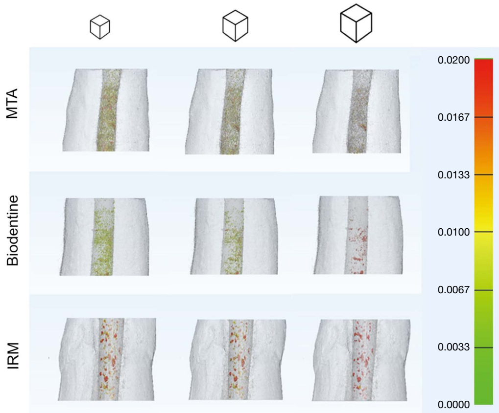
Fig. 3. Three-dimensional models represent the porosity of the MTA, Biodentine, and IRM cements at 5 \mu\text{m} (the small cube represents the smaller voxel size), 10 \mu\text{m} (the medium cube represents the medium voxel size), and 20 \mu\text{m} (the large cube represents the larger voxel size). The color map shows the thickness (mm) of the pores.
