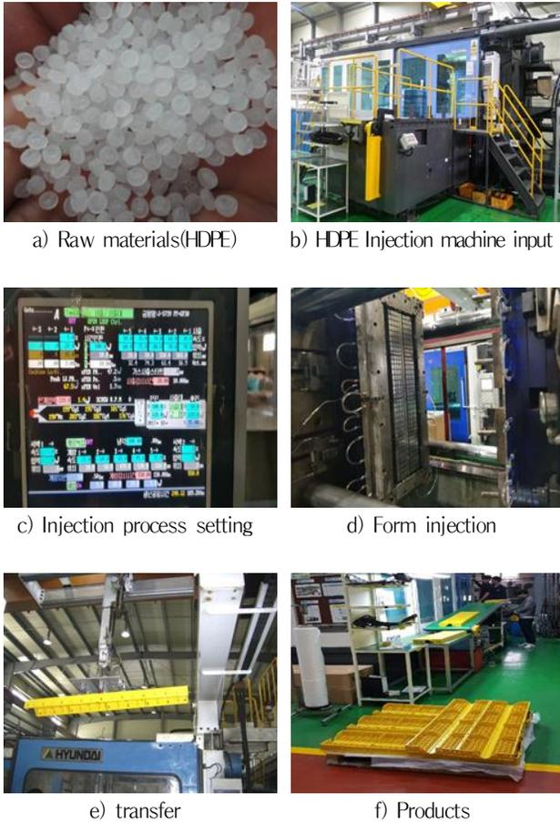
Figure 2. Synthetic resin forming process
