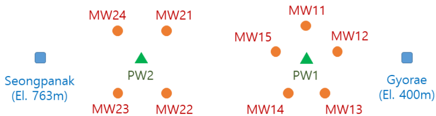
Fig. 1. Schematic diagram of positions of monitoring wells, rainfall stations and pumping wells
