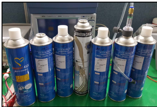
Fig. 5. Standard methane gases and vessels made of six concentrations.
