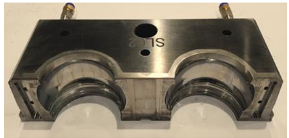
Fig. 10 Slide core completed by vacuum diffusion bonding
