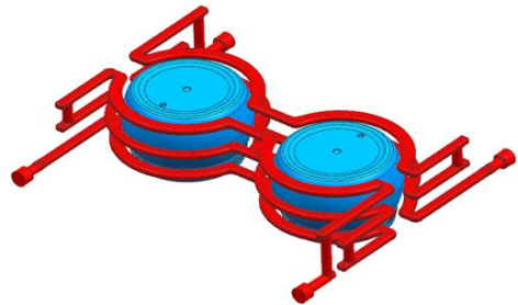
Fig. 7 Configuration of conformal cooling channels designed for tooling slide core
