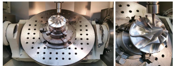
(a) 5-axis machining in AC type machine tool
