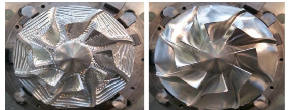
(b) Roughing and finishing by proposed method
