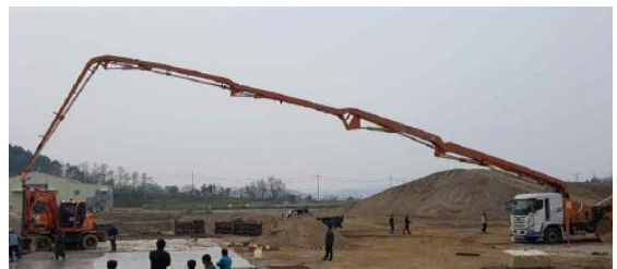
Fig. 12 Pumping test of concrete pump car
