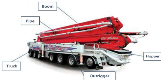
Fig. 1 Concrete pump car
