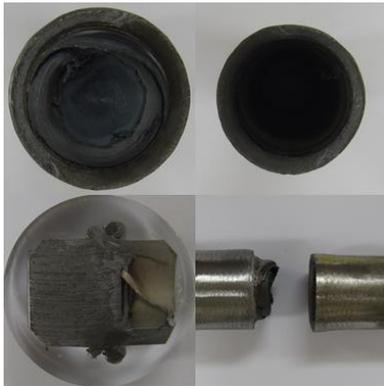
Fig. 6 Fracture shape of tensile specimen
