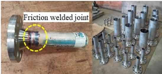
Fig. 1 Shape of piping materials for welded joint
