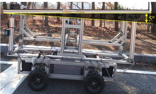
Fig. 11 Ramp movement experiment of the leveling mobile platform
