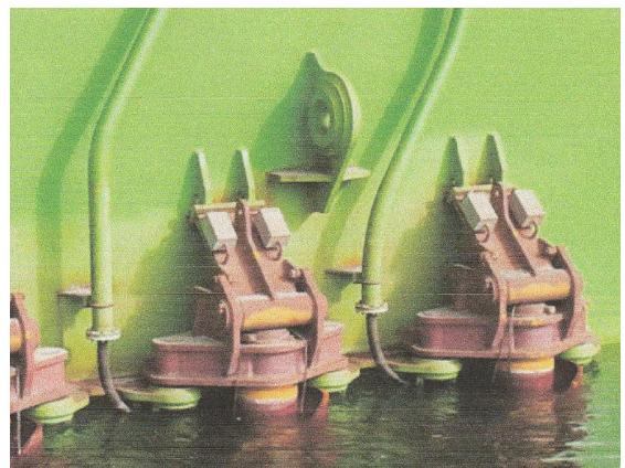
Fig. 7 Photograph of installed cable pipe with cable
