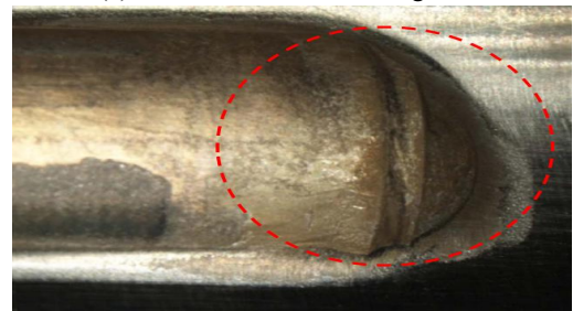
(c) View of the defect on groove
