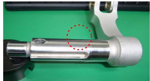
(a) Shape of the similar defected part
