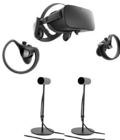
Fig. 2. Oculus Rift HMD, hand-controllers, and two sensors [26]
